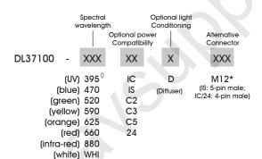
*QUV LEDs have a considerably shorter* half-life than other LEDs (<1000 hrs). For this reason Ai recommends these LEDs be used in strobe mode only. For applications requiring continuous 24v power, contact Ai for assistance.
