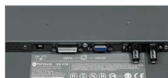
Looping BNC video connector for multiple display connections
