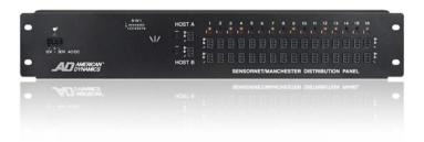
The SensorNet/Manchester distribution panel amplifies either a SensorNet or Manchester protocol signal for multi-point dome control which provides the flexibility to operate efficiently in either protocol setting. With 16 output driver links (two connectors per link), the panel can accommodate home-run dome wiring, multiple daisy-chained links to domes, or J-Boxes.
