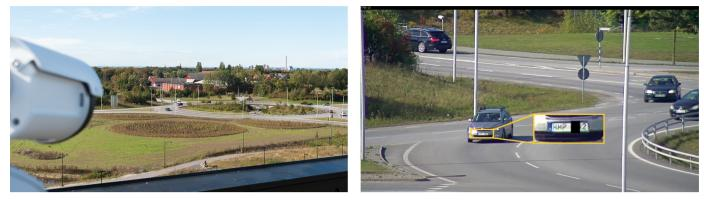
The image to the left is taken with a digital single-lens reflex camera with a 50 mm lens – thus representing the view of the human eye. The image to the right is a snapshot from AXIS Q1765-LE in 18x zoomed-in view where the license plate of a car 275 m (900 ft.) away can be read.
