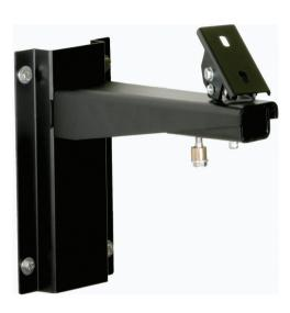
A versatile heavy-duty wall bracket with a dual pin flat plate housing platform has bolt hole arrangements to suit many Extreme CCTV camera housing models. The flat plate is also tilt adjustable with two bolts for secure positioning and single bolt for easy pan positioning. An extra screw slot with bolts allows easy integration with Extreme CCTV illuminators such as the UFLED and SuperLED. EXMB.007 is perfect for solid wall mount applications on various buildings.
