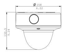
Dimensions in mm (in.) for surface mounting
