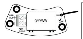
2. Feed your twisted pair wire through the opening at the bottom of the camera body. Attach the twisted pair wires to the terminal block, observing wire color polarity.
