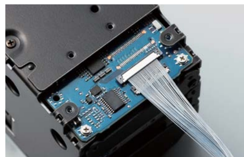
Micro coaxial connector uses KEL CORPORATION's Connector. Pin No.1 is a right edge.
