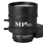
D-YV3.3X15SA-SA2 3 Megapixel Lens 1/3", f:15-50mm, f1.5
