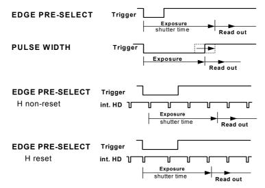
Fig. 8. Trigger modes principle
