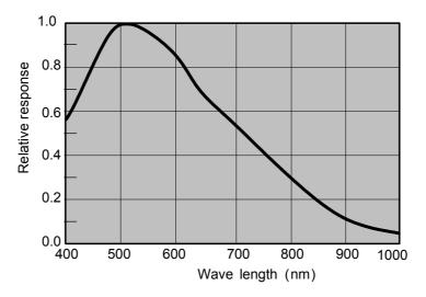
Fig. 26. Spectral sensitivity for CV-M10SX
