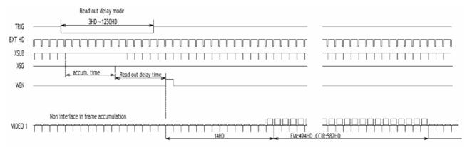
Fig. 18. Frame delay read out. H non-reset
