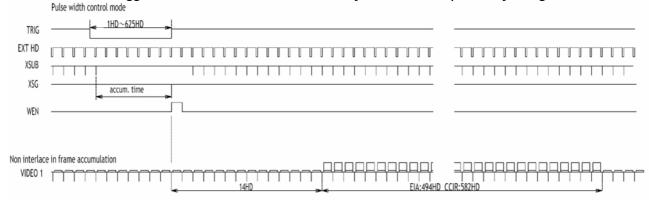
Fig. 16. Pulse width control. H non-reset
