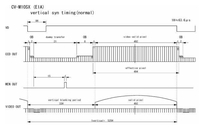
Fig. 12. Vertical timing EIA
