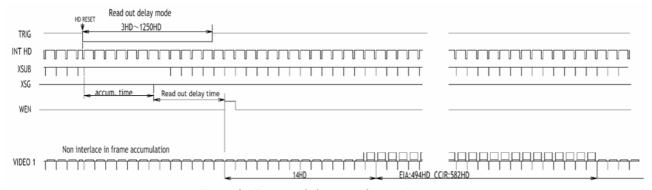
Fig. 19. Frame delay read out. H reset
