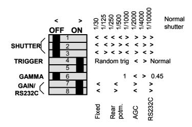
**Note:** The shown switch settings are the factory setting. Values are shown for EIA.
