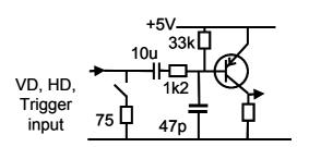
Fig. 5. HD, VD and Trigger input.
