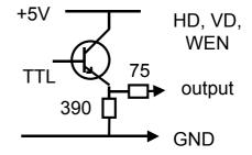
Fig.6. HD and VD input.
