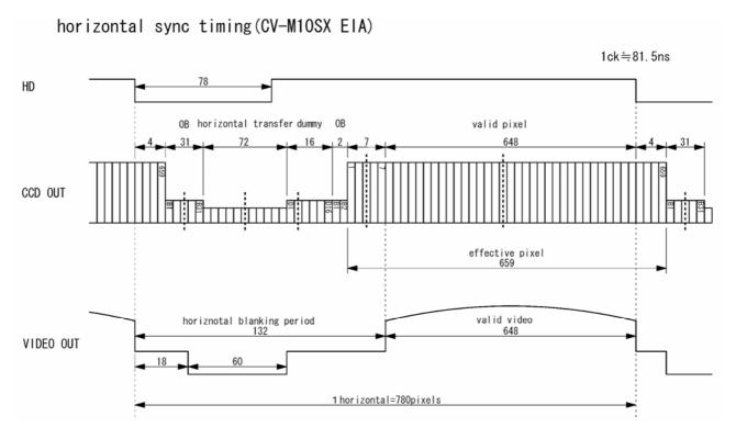
Fig. 10. Horizontal timing EIA
