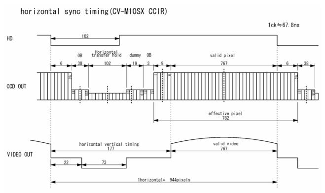
Fig. 9. Horizontal timing CCIR
