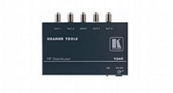
The 104R is a high-performance distribution amplifier for analog RF signals. It takes one RF (CATV/MATV) signal and distributes it to four identical outputs.
