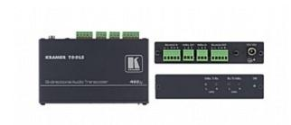
The 482xl is a high-performance audio transcoder for balanced and unbalanced stereo audio signals. It simultaneously converts balanced stereo signals to unbalanced stereo audio and unbalanced stereo audio signals to balanced stereo audio.
