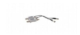
The 613R/T is a receiver/transmitter pair for digital video signals up to 3G HD-SDI. The 613T converts the digital signal into an optical signal that it transmits over single-mode fiber optic cable and the 613R decodes the optical signals back to the original digital format video signal.
