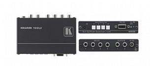
The 6502 is a high-performance switcher for S/PDIF digital audio signals. The unit takes any one of four inputs, provides reclocking and equalization and distributes the signal to two identical outputs.
