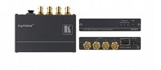
The 673T and 673R are a high-performance fiber optic transmitter and receiver for video signals up to 3G HD-SDI and dual link HD-SDI signals. The 673T converts up to four channels of SDI signals on BNC connectors to an optical signal that is transmitted over a single fiber optic cable. The 673R converts the optical signal back to SDI signals.
