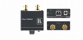
The 690R is a high-performance fiber optic receiver for SDI video signals up to 3G HD-SDI. The 690T converts two 3G HD-SDI signals to single-mode fiber optic and the 690R receiver converts them back to the two original SDI formats. Compatible with the fiber optic matrix VS-88FO.
