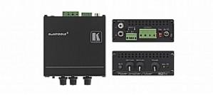
The 907xl is a high-performance power amplifier for line-level stereo audio signals. It accepts a balanced stereo audio signal on a terminal block connector and an unbalanced stereo signal on RCA connectors. It delivers 40 watts per channel into an  $8\Omega$  load.
