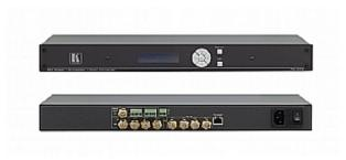
The FC-340 is a broadcast-quality video scaler, audio embedder/de-embedder and scan converter for digital video signals up to 3G HD-SDI. The unit inputs an SDI signal and simultaneously outputs SDI and composite video signals while the audio embedded in the SDI input signal is output to both AES/3id and balanced audio outputs.
