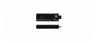
The KW-11T and KW-11R is a high-definition, wireless, HDMI transmitter and receiver combination for indoor use over short range distances. The KW-11T converts an HDMI signal into a wireless signal that it transmits to the KW-11R. The KW-11R converts the wireless signal back into HDMI.
