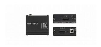
The PT-101DP is a repeater for DisplayPort video signals. The unit reclocks and equalizes the signal and can extend the length of a DisplayPort line up to a combined length of 35m (115ft) at resolutions of UXGA/1080p using Kramer cables. Multiple units can be cascaded.
