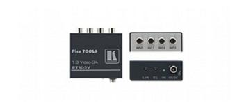
The PT-103V is a composite video distribution amplifier. It takes one input, provides correct buffering and isolation and distributes the signal to three identical outputs.
