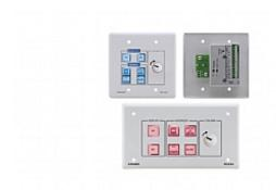
The RC-63AL is a 6-button room controller with an analog volume knob for multimedia rooms. The unit can control audio components, video components and other room facilities such as lights and screens.
