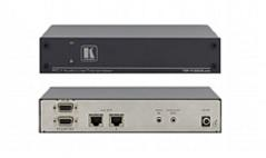
The TP-100AXR is a twisted pair transmitter for computer graphics video and unbalanced stereo signals. The TP-100AXR converts the input signals into a twisted pair signal and the TP-200AXR converts the twisted pair signal back into two computer graphics signals, as well as two stereo audio plus two S/PDIF audio signal.
