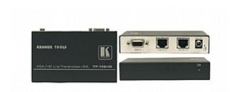
The TP-102HD is a twisted pair transmitter for computer graphics video and HDTV signals. It converts a computer graphics video or HDTV signal on a 15-pin HD connector to two identical twisted pair signals.
