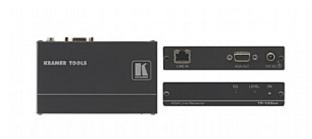
The TP-120-od is a twisted pair receiver for computer graphics video signals. When used in conjunction with the PT-110-od twisted pair transmitter (or other compatible Kramer transmitter), it converts a twisted pair signal back into a computer graphics video signal.
