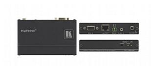
The TP-123-od is a high-performance twisted pair transmitter for computer graphics video, unbalanced stereo analog audio and unidirectional RS-232 control command signals. It converts the input signals to a twisted pair signal and transmits it over twisted pair cable to a TP-124-od receiver.
