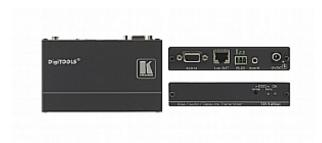
The TP-125xl is an extended range twisted pair transmitter for computer graphics video, unbalanced stereo audio and bidirectional RS-232 control command signals. It converts the input signals to a twisted pair signal and transmits them over CAT 5 cable to a compatible receiver.
