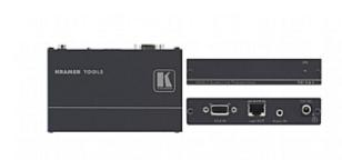
The TP-141 and TP-142 are an extended range twisted pair transmitter and receiver for computer graphics video (including HDTV) and unbalanced stereo audio signals, with high electrical noise immunity. The TP-141 converts computer graphics video and audio inputs to twisted pair signals, and the TP-142 converts the twisted pair signals back into computer graphics video, unbalanced stereo and S/PDIF digital audio signals.
