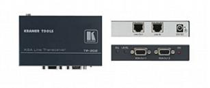
The TP-202 is a twisted pair branching receiver for computer graphics video signals with resolutions up to and exceeding UXGA or HDTV signals. It takes a twisted pair signal and converts it into a computer graphics or HDTV signal available on two 15-pin HD outputs, and simultaneously re-transmits the original twisted pair signal to another compatible receiver.
