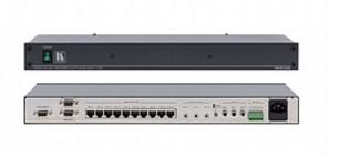
The TP-210A is a high-performance distribution amplifier and twisted pair transmitter for computer graphics video signals with resolutions up to UXGA, RS-232 signals and stereo or S/PDIF audio signals. The unit takes computer graphics video, stereo or S/PDIF audio and RS-232 signals and distributes each signal to two local outputs and ten twisted pair outputs.
