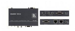
The TP-50 is a twisted pair receiver for computer graphics video and unbalanced stereo audio or S/PDIF audio signals. The unit converts the twisted pair signal back into two computer graphics video, stereo audio and S/PDIF audio signals simultaneously.
