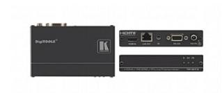
The TP-573 is a DGKat™ twisted pair transmitter for HDMI, bidirectional RS-232 and infrared signals. The TP-573 converts the input signals to a twisted pair signal and the TP-574 converts it back to HDMI, RS-232 and infrared signals.
