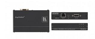
The TP-574 is a DGKat™ twisted pair receiver for HDMI, bidirectional RS-232 and infrared signals. The TP-573 converts the input signals to a twisted pair signal and the TP-574 converts it back to HDMI, RS-232 and infrared signals.
