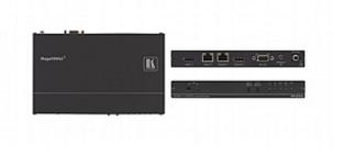
The TP-576 is a DGKat<sup>™</sup> twisted pair line driver for HDMI, bidirectional RS-232 and infrared signals. The unit receives an HDMI signal either from a local HDMI source or from a compatible twisted pair transmitter. It decodes the selected signals to the local HDMI, RS-232 and IR outputs and simultaneously transmits them to a compatible twisted pair receiver.
