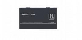
The TR-1YC is a high-performance isolation transformer for s-Video (Y/C) signals. It provides complete isolation between devices to eliminate hum, ground loops and DC offsets, which can degrade the video quality.
