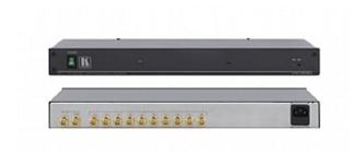
The VM-10HDxl is a high-performance distribution amplifier for 3G HD-SDI signals. The unit takes one input, provides reclocking and equalization and distributes the signal to ten identical outputs.
