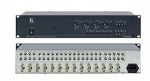
The VM-20ARII is a multi-format, high-performance distribution amplifier that can also be configured for composite video and unbalanced stereo audio signals. It can be configured as a 1:10 distribution amplifier for s-Video (Y/C) signals or a 1:5 distribution amplifier for RGBS signals, both with unbalanced stereo audio.
