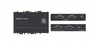
The VP-222K is a high-performance switcher for computer graphics video signals with resolutions up to and exceeding UXGA. It switches one of two inputs to two identical outputs.
