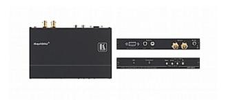
The VP-483 is a high-performance digital scaler for computer graphics video signals to WUXGA and 1080p and stereo audio. The unit embeds the audio and up or down scales input to two SDI, HD-SDI or 3G HD-SDI signals.
