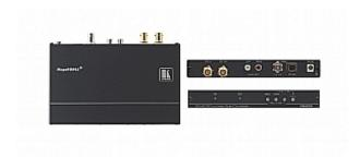
The VP-505 is a high-performance scan converter for digital video signals up to 3G HD-SDI. The unit de-embeds the audio to unbalanced stereo audio and down-scales the video to composite and s-Video (Y/C) simultaneously in either PAL or NTSC formats.
