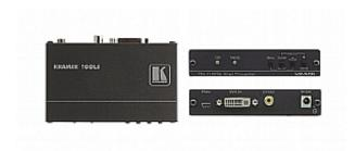
The VP-506 is a high-quality scan converter for down-scaling DVI, computer graphics (VGA) and component video (YPbPr) to PAL or NTSC video. It supports VGA up to UXGA, as well as component resolutions up to 1080p.
