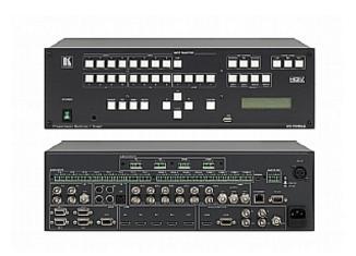
The VP-725NA is a presentation scaler/switcher with multiple signal format sections and balanced stereo audio. The unit has five independent 4x1 video sections: composite, s-Video (Y/C), component (YUV), computer graphics and HDMI, plus a single USB input. It also scales any video input up or down to a selectable graphics or HDTV output resolution and provides glitch-free switching between sources through FTB™ (fade-thru-black) switching technology.
