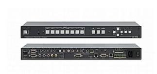
The VP-770 is a high-performance presentation switcher and scaler for composite video, component video, DisplayPort, computer graphics video, and HDMI signals. It scales the video, embeds the audio and outputs the signal to HDMI, computer graphics and DGKat twisted pair, together with digital audio, unbalanced stereo and a 10-watt amplified balanced stereo speaker output.
