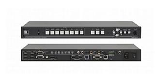
The VP-773 is a high-performance presentation switcher and scaler. It accepts one of eight inputs: one DisplayPort (DP), one composite video, two computer graphics and four HDMI signals. It scales the video, embeds the audio, and simultaneously outputs the signal to two HDMI and one HDBaseT TP output, together with S/PDIF and balanced stereo audio outputs.
