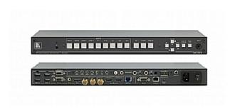
The VP-774 is a high-performance presentation switcher and scaler. It accepts one of nine inputs: one 3G HD-SDI, one DisplayPort (DP), one composite video, two computer graphics and four HDMI signals. It scales the video, embeds the audio, and simultaneously outputs the signal to two HDMI, one SDI and one HDBaseT TP output, together with S/PDIF and balanced stereo audio outputs.
