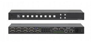
The VP-81KSi is a high-performance analog step-in switcher for computer graphics video with resolutions up to WUXGA and unbalanced stereo audio signals. The unit can switch any one of eight inputs to one computer graphics video, one unbalanced and one balanced stereo audio and one twisted pair output. The VP-81KSi works in conjunction with up to eight VGA Remote Control Step-in Modules including the SI-1VGA (for TBUS-10), SI-VGAT (under the table) and WSI-1VGA (for standard TBUSes).
