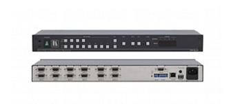
The VP-8x4 is a high-performance matrix switcher for computer graphics video signals, with resolutions up to and exceeding UXGA. It can route any or all of its eight inputs to any or all of its four outputs simultaneously.
