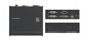
The VS-21HDCP-IR is a high-quality switcher for DVI signals. It equalizes the signal and switches either of two inputs to a single output.
