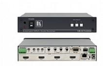
The VS-311H is a high-performance switcher for HDMI video and balanced, unbalanced and S/PDIF audio signals. When configured as a standby switcher, it switches to a selectable secondary input upon loss of the primary input.
