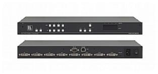
The VS-44HDCP is a high-quality, HDCP compliant 4x4 DVI matrix switcher. It reclocks and equalizes the signals and can route any of the four DVI/HDMI (over DVI–I connectors) inputs to any of the four DVI/HDMI outputs simultaneously.
